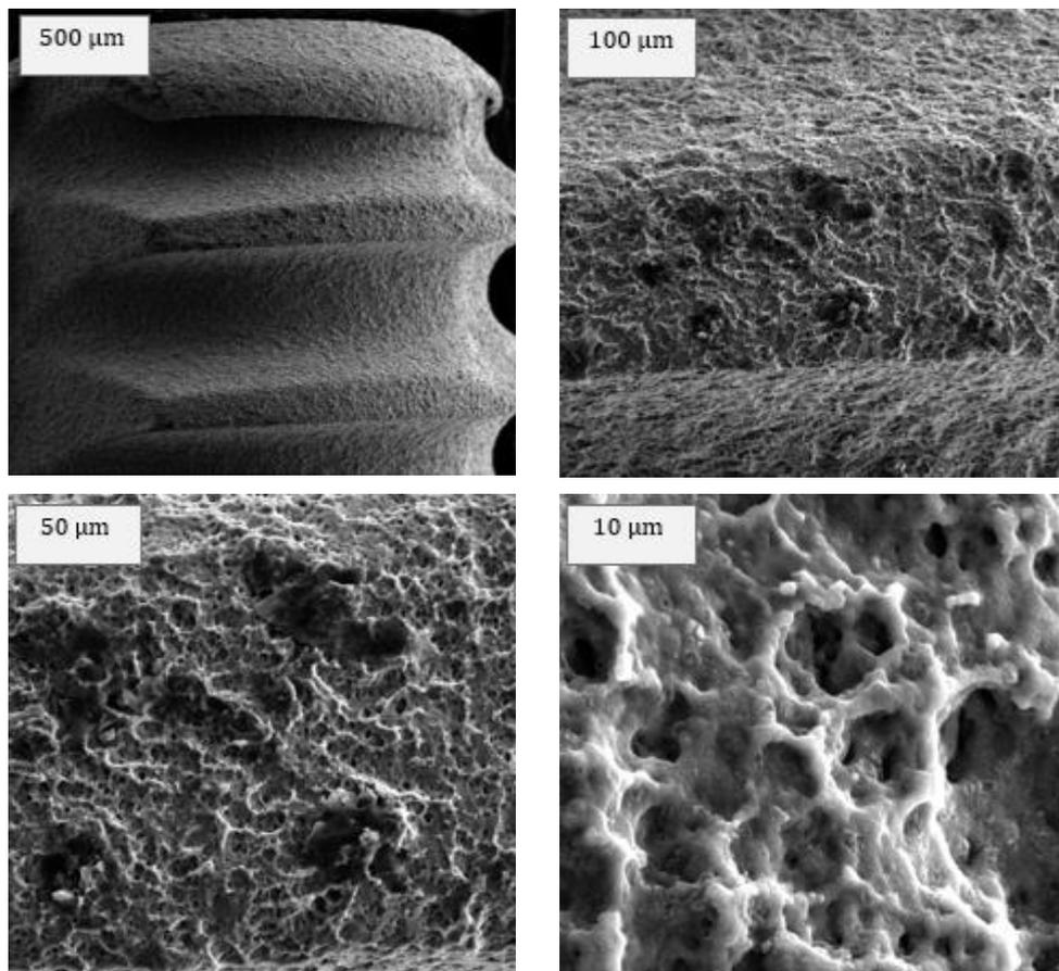
**Fig.4. SEM images related to SLActive surface treatment method for 3A titanium implant fixture**
