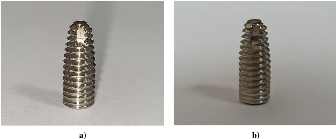
**Fig.1. Implant fixture 3A a) before and b) after sandblasting operation and acid etching**
