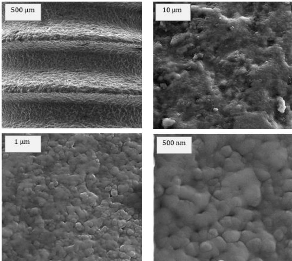
**Fig.3. SEM images related to SLA surface treatment method for 3A titanium implant fixture**
